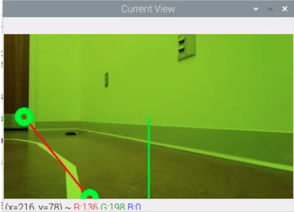
Figure 9: Relative heading and offset of track in camera coordinates
