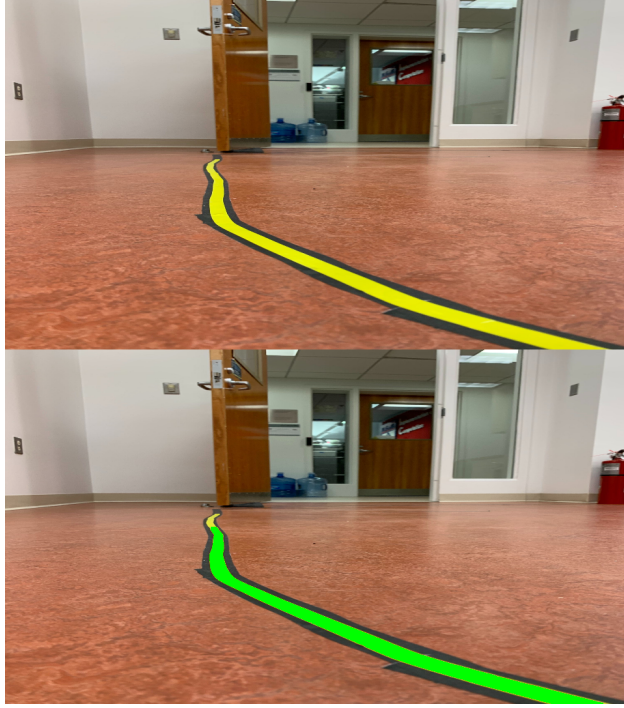
Figure 8: The top photo is the original unaltered track. In the lower photo, the detected track is highlighted in green. Note that the picture is cropped during detection to avoid artifacts in the horizon, hence the failure to detect the later track.
