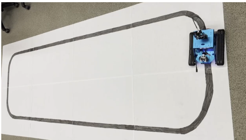
Figure A4: Original robot using line tracking to follow a prescribed track
