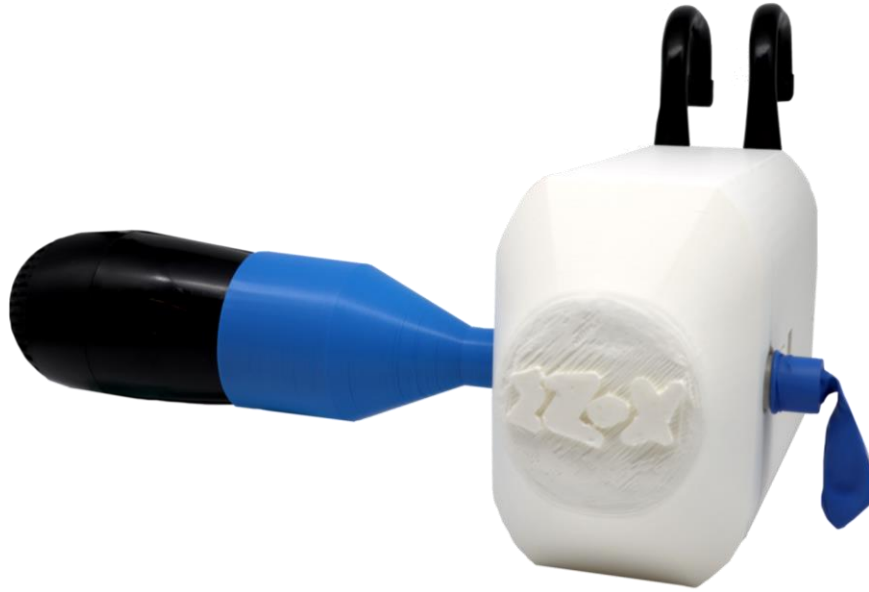
Figure 11: The EZ-X testing mechanism comprising a hair drier to replicate the airflow patterns of a ventilator (left), the EZ-X device itself (center), and a balloon to simulate pressure build up, similar to that of a lung (right).
