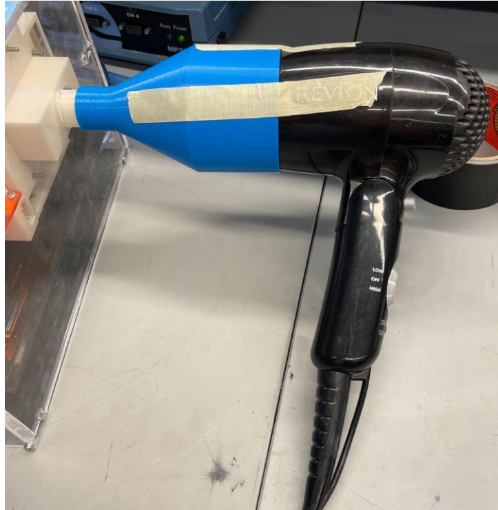
Figure 9: Pictured above is a Revlon hair dryer, used to replicate a mechanical ventilator input to the EZ-X device. This includes a special attachment (in blue) to allow for proper connection to the input side of the device.
