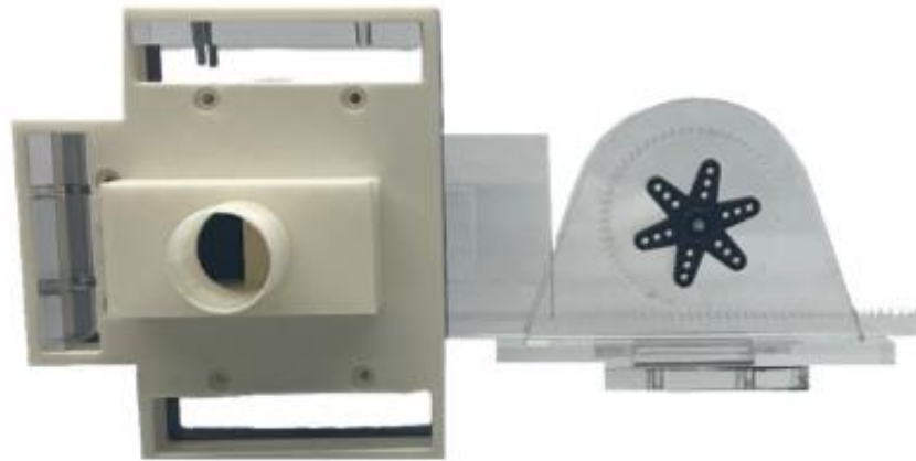
Figure 3: Rack and Pinion based mechanical valve built for MVP
