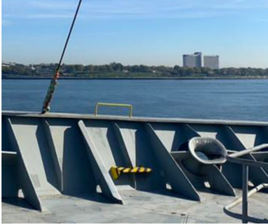
Fig. 2. Anchor-watch's footing, where they lean out to see the chain
