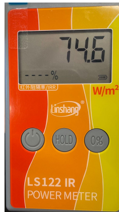
Figure 8. A representative reading of Infrared Therapy on LS122 IR Power Meter at 74.6 W/m 2 . The reading was consistently around 75 W/m 2 , meeting the technical specification of 50 W/m 2 .
