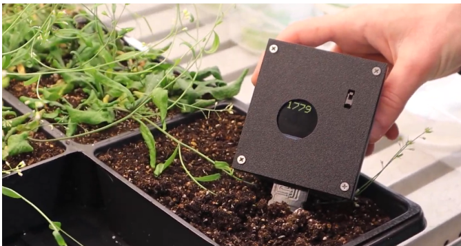
Figure 11: Example Greenhouse Setup With Capacitance Soil Sensors on Custom Built Testing Hardware
