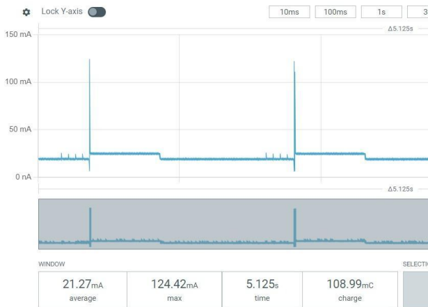
Figure 13: Empirical Measurements of Current Through Active RF Transmissions on The Peripheral Hardware
