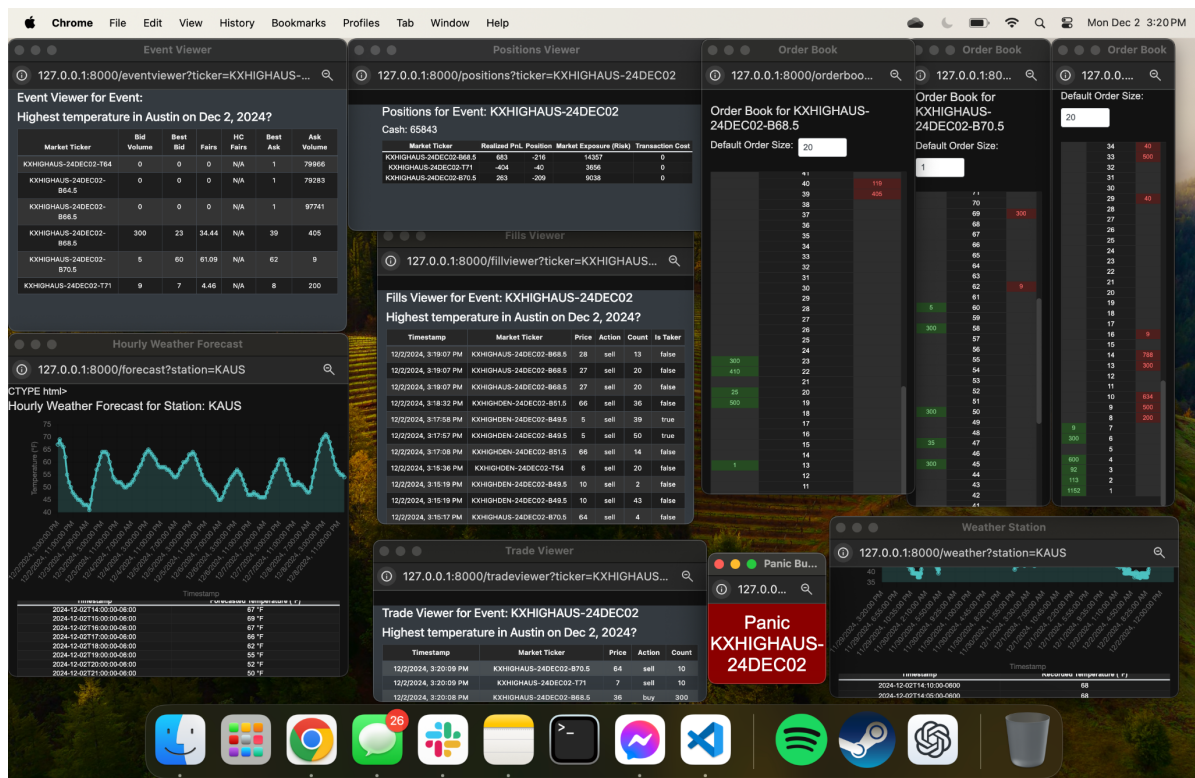
Figure A.1: A manual trading set up showing our event viewer, trade viewer, fills viewer, orderbook viewer (where the user can place orders), primitive positions viewer, and weather charting
