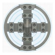
This is because our edge cutters scrape away more than the diameter of our tunnel to produce an industry-standard overcut. The extent of this overcut is a  $\frac{1}{2}$ " thick ring. This puts the effective cut diameter to 21".
