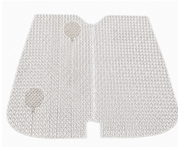
Figure 14: Foam-TPU flexible garment segment for the upper arm.
