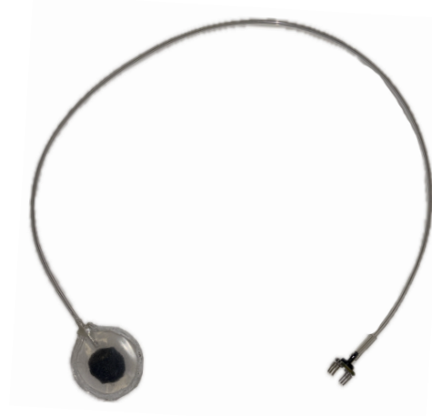
Figure 4: Assembled pressure pouch sensor.
